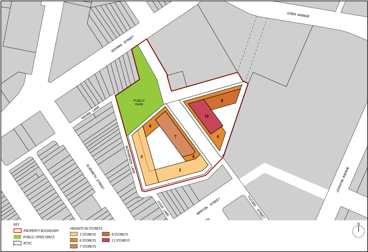
Figure 6.xx: 904 Bourke Street, Zetland – Building heights in storeys
